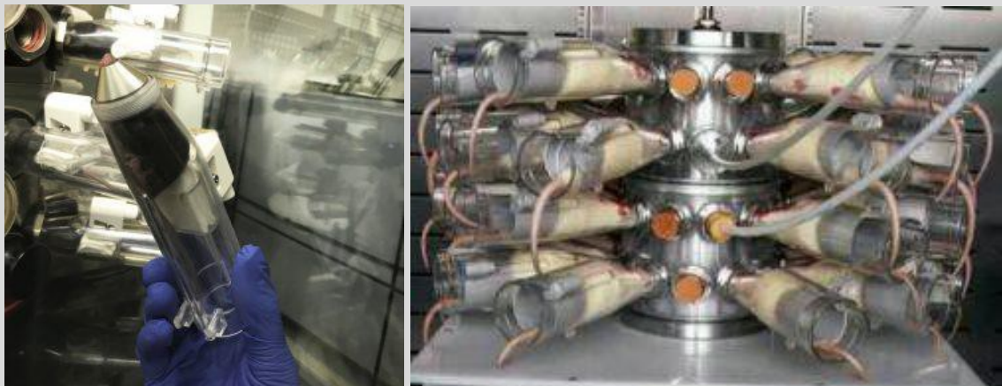
Figure 2 nose-only exposure of mice to inhalants in a 'smoking tower'
